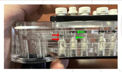
After shutting off product flow to the handle, if the soda and/or water buttons are operating appropriately, the technician may press down on those buttons and test for "spring back" on the syrup buttons around the water/soda. All syrup buttons should spring back up to the closed position by themselves while pressing down the soda/water button they are connected to.
